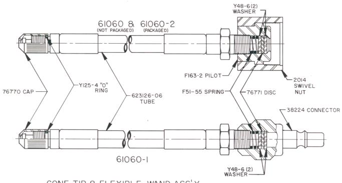
CONE TIP & FLEXIBLE WAND ASS'Y. (HIGH PRESSURE)
